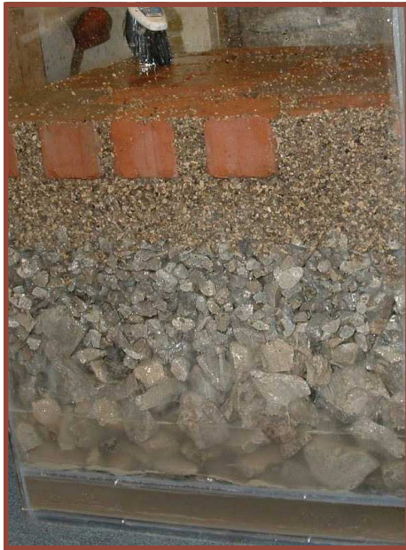
Eifert built a demonstration model to show how quickly water percolates through the brick paver road system.
